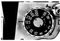
5 If the meter needle is pointing above the meter index and cannot be matched by closing the preset aperture ring and metering cannot be performed, turn the shutter speed dial to the faster side. If the meter needle is pointing below the meter index and cannot be matched by opening the preset aperture ring, turn the shutter speed dial to the slower side. When the red signal appears, use high-speed film or the Canon Booster.
